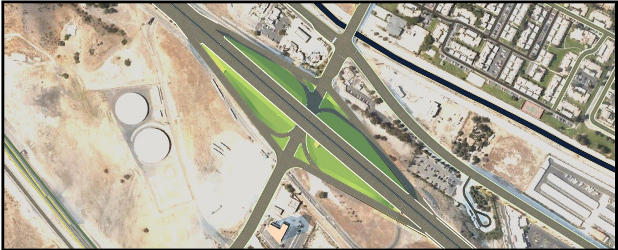
Figure 4: Single Point Interchange design alternative.
